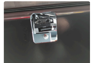
Fill level sensor viewed from inside the bin
